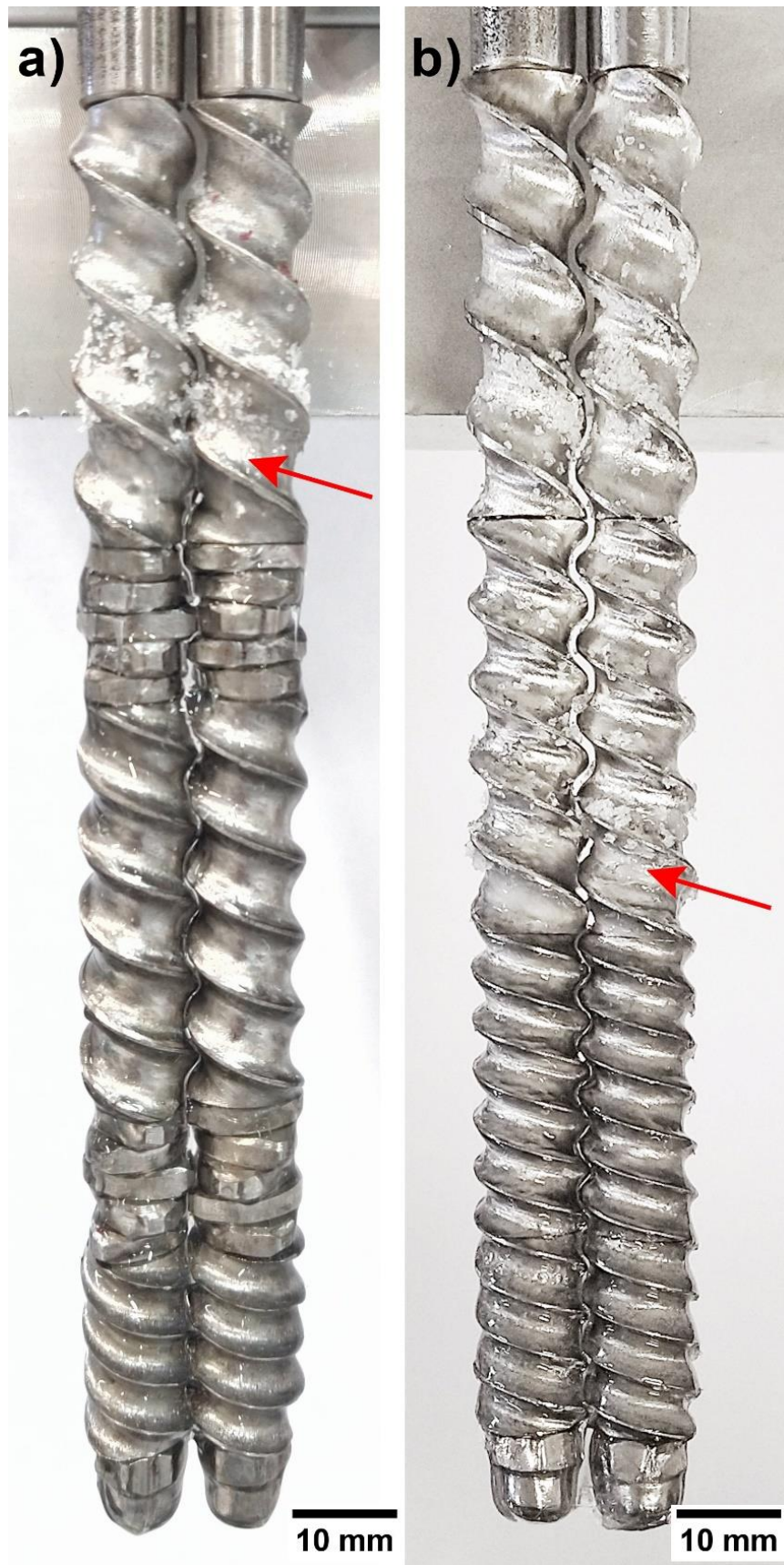
Figure 67. Screw pull-out experiments evidencing the influence of the screw configuration on the melting location: (a) configuration 1; (b) configuration 2.
