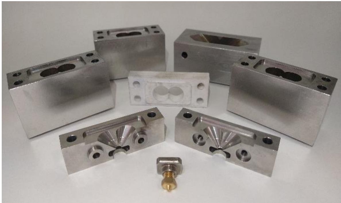
Figure 62. Barrel modules, insulating PTFE segment and threaded sleed with the deposition nozzle.
