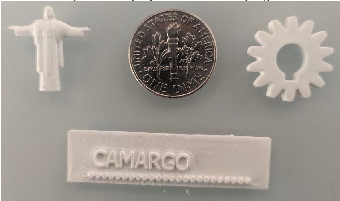
Figure 45 – 3Y-TZP green parts manufactured in the built prototype.
