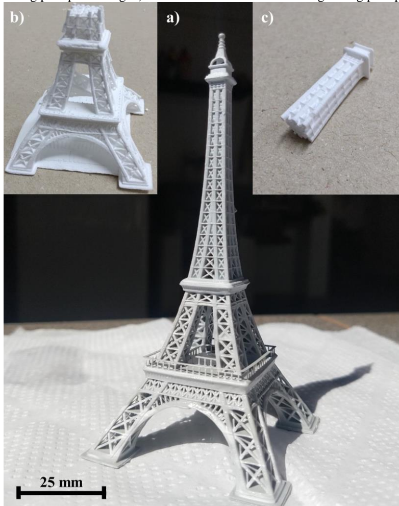
Figure 65 – Mullite 3D printed part with tiny structures. a) Green part (Eiffel Tower). b) Base of the tower after breaking during post-processing. c) Piece of the tower after breaking during post-processing.
