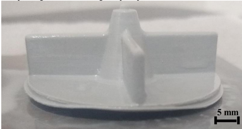
Figure 62 – 3D printing fail of a mullite green part: partial detachment from the build platform.
