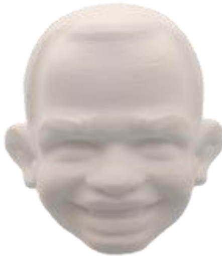
Figure 81 – 3D caricature of the author of this thesis made of mullite (3D model created by the artist Raul Tabajara, manufactured from the 40 vol% mullite suspension in the selected commercial 3D printer and sintered at 1600 °C)
