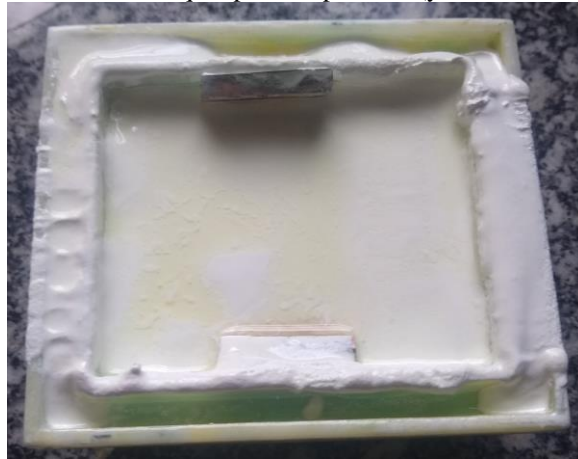
Figure 36 – Ceramic suspension based on preliminary studies of our research group, after 4 hours of preparation, presenting sedimentation and liquid phase separation (yellowish coloring) at the top.
