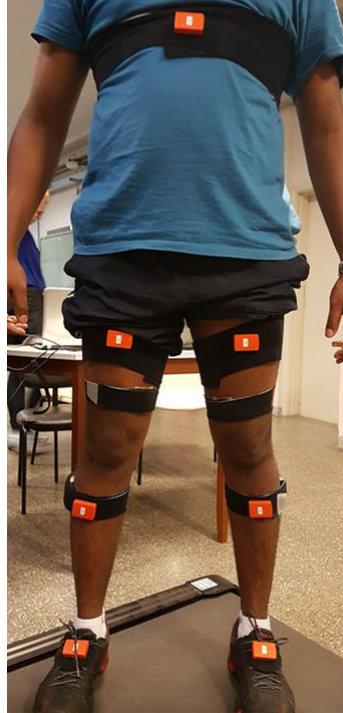
Figure 22 – IMUs on the user’s torso, thigh, shin and foot.
