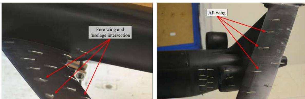
Figure 40 – Mini-tuft flow visualization on the wing surfaces at M = 0.089 , Re = 3.02 \times 10^5 , and \alpha = 10^\circ .
