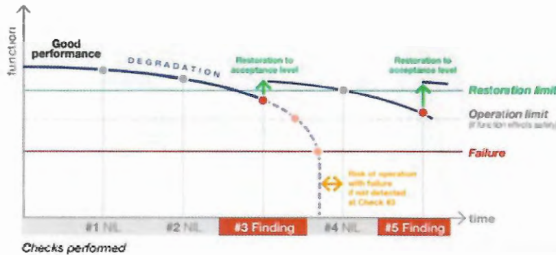
Figure 2 – Functionality vs. Time for a preventively maintained metallic component.
