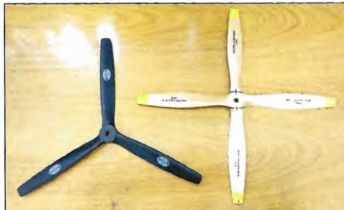
Figure 60 – 3-Bladed 16" x 8" propeller and 4-Bladed 16" x 6" propeller
