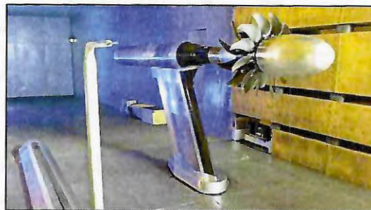
Figure 27 – Open rotor rig with historical baseline blades
