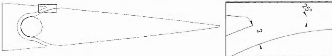
Figure 71 – Shape of the pylon trailing edge with integrated blowing system
