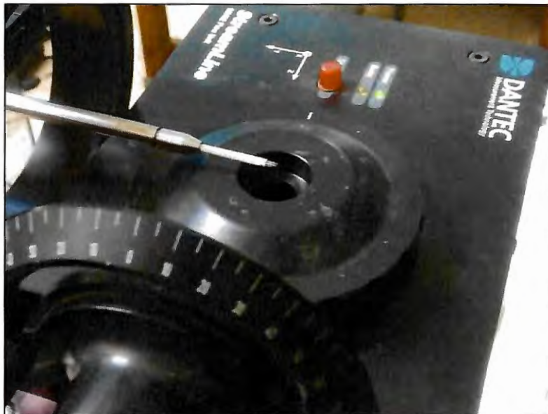
Figure 157 – Calibration of the hot-wire probe
