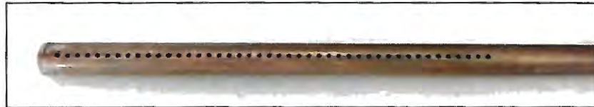
Figure 74 – Drilled cylinder for feeding air to the blowing slots
