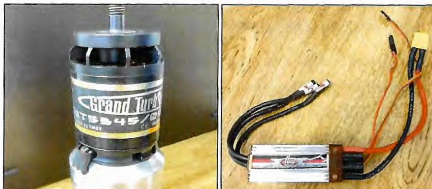
Figure 61 – Electric motor and ESC for the propeller operation
