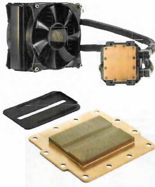
Figure 1.3 – Commercial heat sink for CPUs based on microchannels and using water as the working fluid. Model Nepton 140XL from Cooler Master
