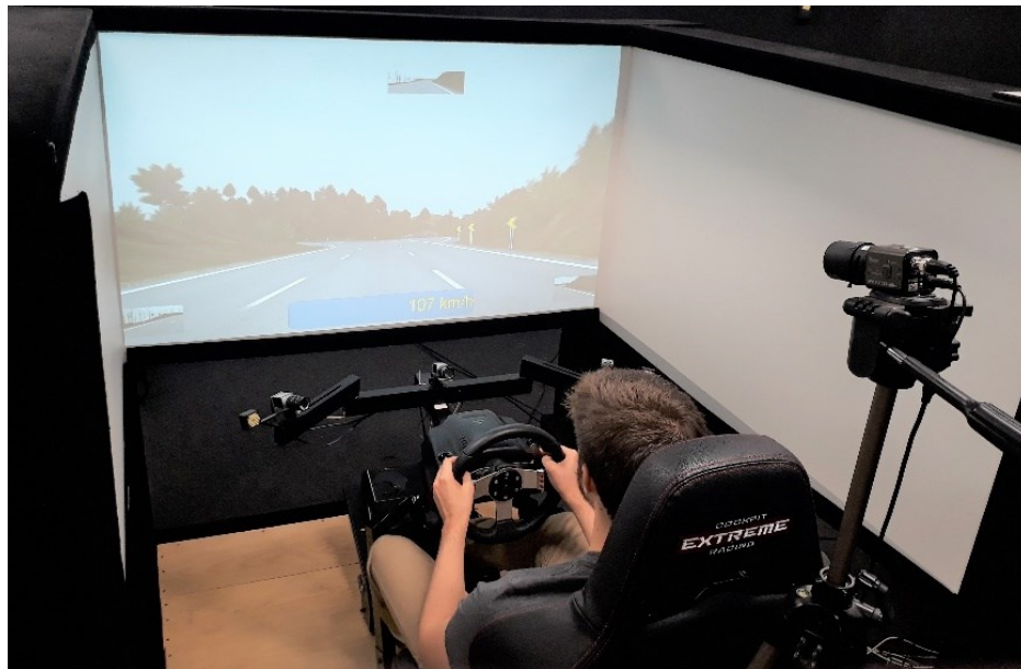
Figure 1 – Simulator's physical structure
