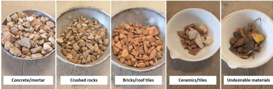
Figure 11: Composition of recycled masonry aggregates.
