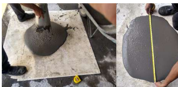
(e) Slump test do UHPFRC
