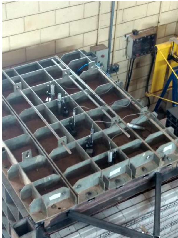
Figure 5.77: Displacement transducers installed at the model wall (passing through the box lid) to measure soil settlement.
