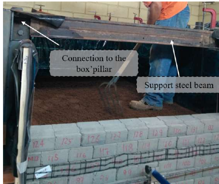
Figure 5.12: Steel front support beam bolted to the front box pillars.
