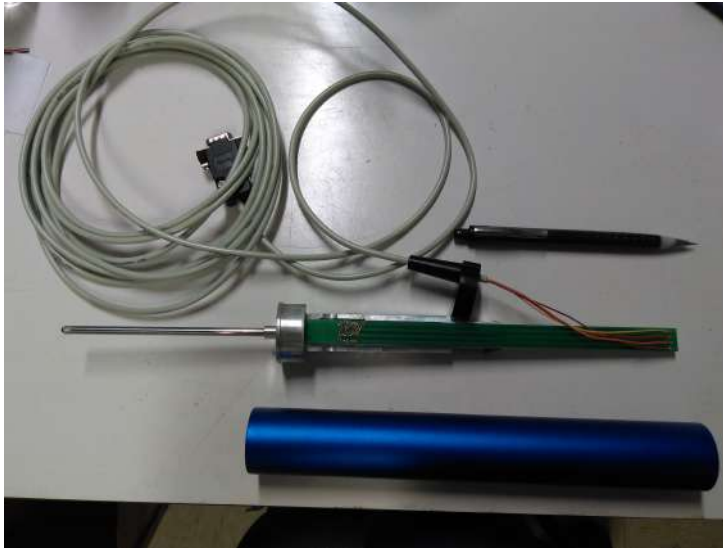
Figure 5.35: Displacement transducer mounted.
