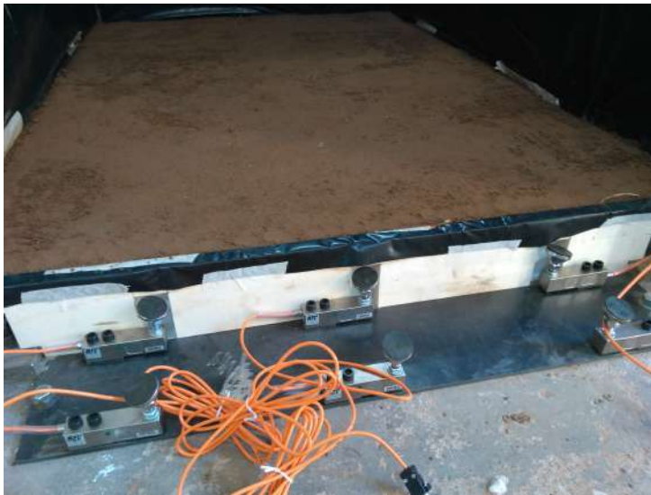
Figure 5.54: Vertical load cells screw-mounted on the base plate of the toe set-up.
