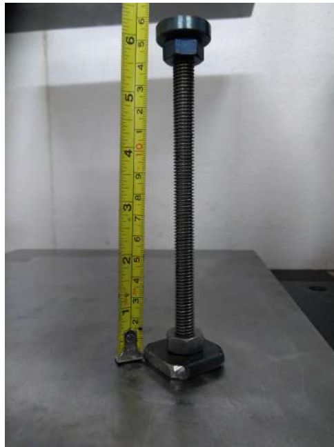
Figure 5.31: Steel rod adapted to support the displacement transducers to measure soil surface settlement.
