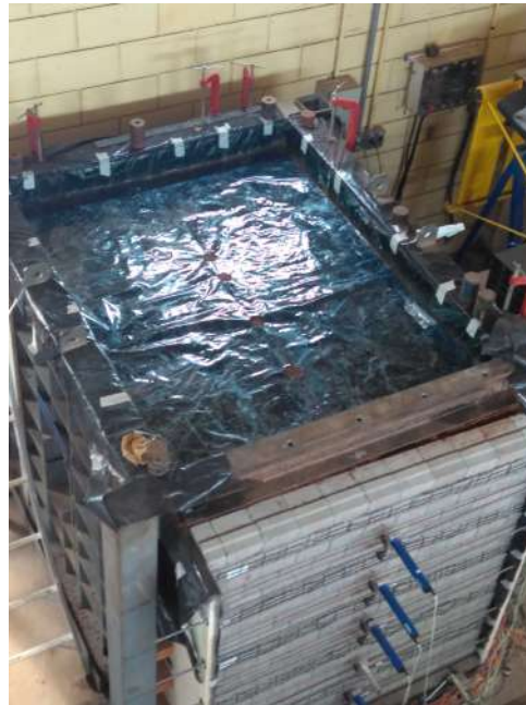
Figure 5.20: Soil top surface covered with friction reducing membranes.
