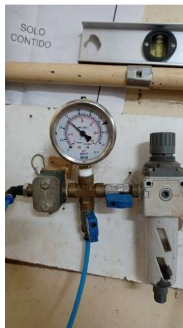
Figure 5.24: Pressure panel used to control the air inflow and pressure to each airbag.
