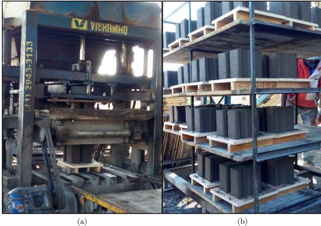
Figure 5.9: Reduced-scale modular block facing units: a) manufacturing process; b) block cure; c) block storage at LabGsy laboratory.
