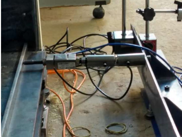
Figure 5.56: Horizontal toe load cell mounted between the stiff reaction beam and the flap at the facing block base plate.
