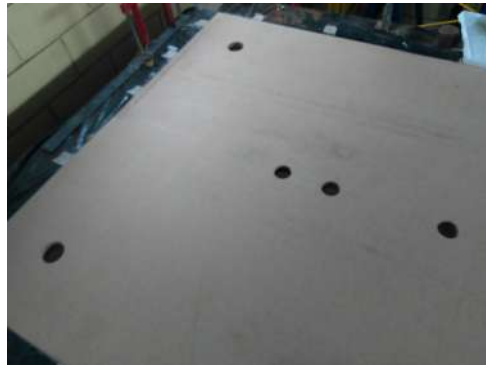
Figure 5.22: Plywood board placed over the airbag + geotextile set-up.
