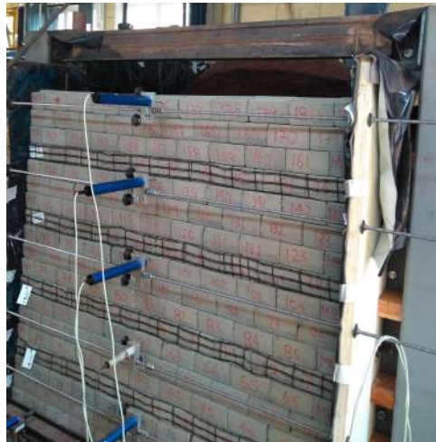
Figure 5.27: Displacement transducers support during wall construction: fixation on transversal tie rods.
