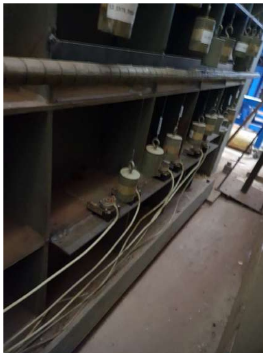
Figure 5.43: Weight system attached to extensometer wire end.
