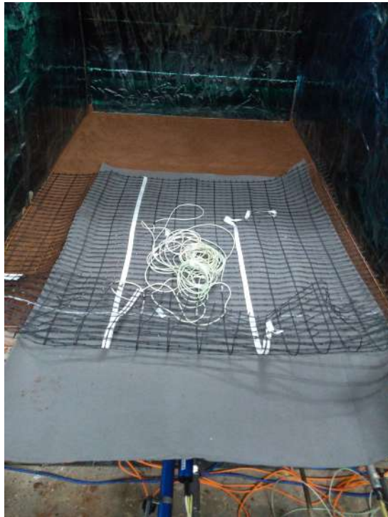
Figure 5.72: Geogrid placement at the backfill soil by using an geotextile sheet.
