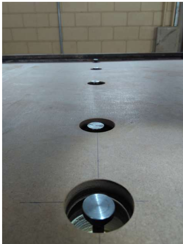
Figure 5.78: Rod adapters installed inside the pre-drilled holes at the plywood and MDF boards of the surcharging set-up.
