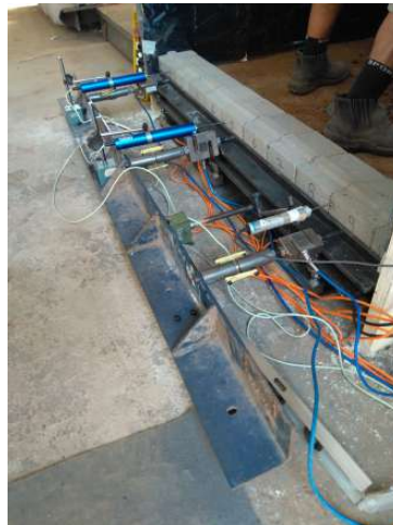
Figure 5.30: Toe instrumentation: displacement transducers and load cells.
