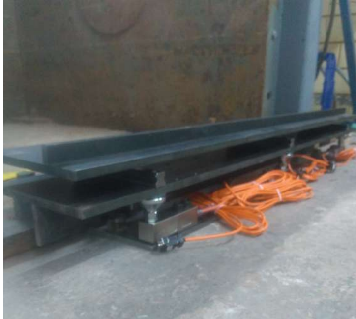
Figure 5.55: Toe set-up: base plate with vertical toe load cells (bottom), middle plate with linear bearings and facing block base plate (top).
