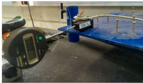
Figure 5.44: Calibration of the draw-wire potentiometers.
