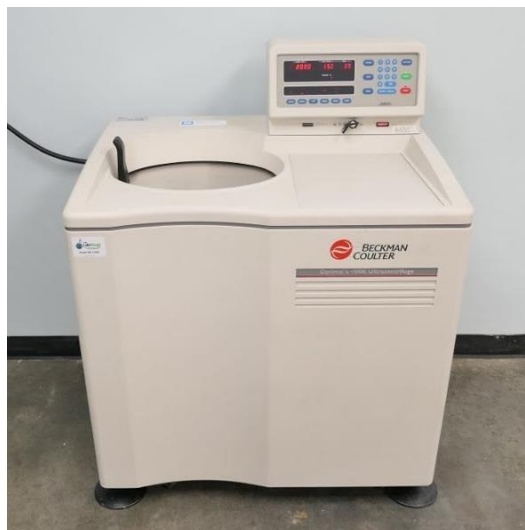
Figura 5. Ultracentrífuga Optima L-100K Beckman Coulter (Fonte: The Lab World Group, disponível em: https://www.thelabworldgroup.com/product/beckman-coulter-optima-l-100k-ultracentrifuge/ )
