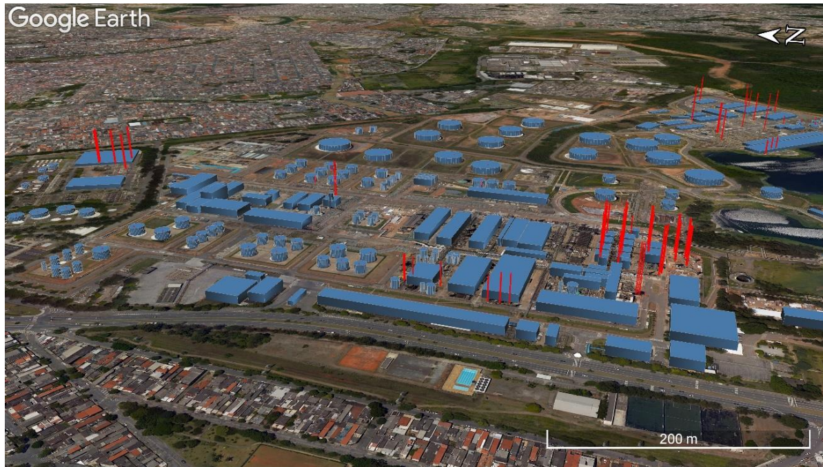
Figure 3.2. Braskem and RECAP industrial plants on tridimensional modeling. In blue are the buildings or tanks, in red are the point sources (stacks/flare). Source: Google Earth (accessed on 11 March 2023)
