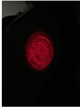
Figure 3.2: Annulus pattern in far field illumination yielded by a misaligned fiber in the lab. Experiment made in IAG lab.
