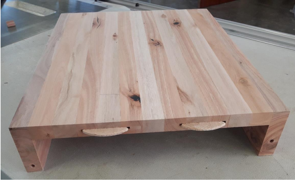
Figure 3. Detail of the connections used: biscuit joints at the top and dowel connections at the bottom on both sides.
