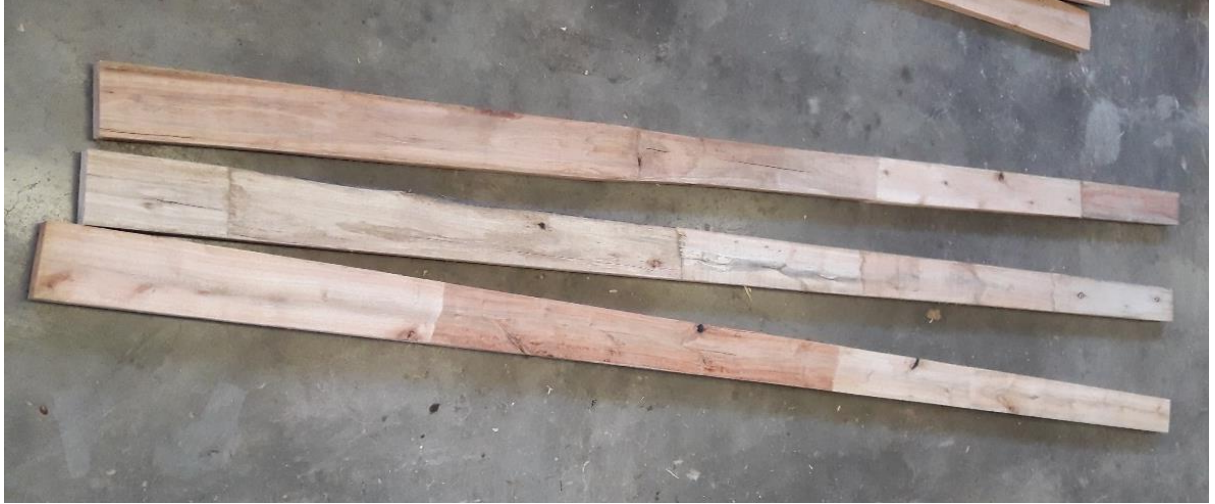
Figure 38. Raw material: finger-jointed boards of young Eucalyptus grandis timber.
