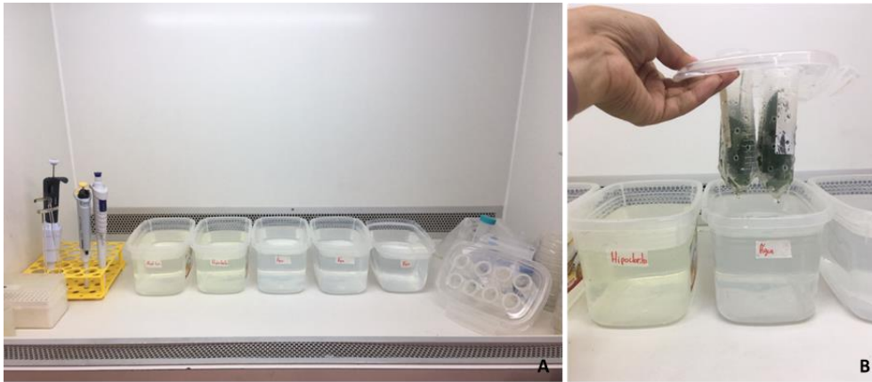
Figure 5. Bulk surface-sterilization. Material to realize the bulk surface-sterilization with the sequence of 70% ethanol, sodium hypochlorite and three times of sterile water (A). Surface sterilization leaves with Falcon tubes adapted according to the methodology (B).
