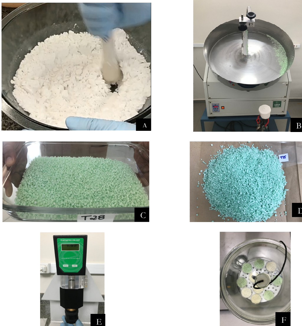
Suppl. Figure 1. Urea mixture with molybdenum trioxide for granulation (A); Fertilizer granulation (B); Preparation for fertilizers drying (C); Mixture formulated before the granules are separated by size (D); Evaluation of granule hardness (E); and evaluation of the fertilizers hygroscopicity (F).
