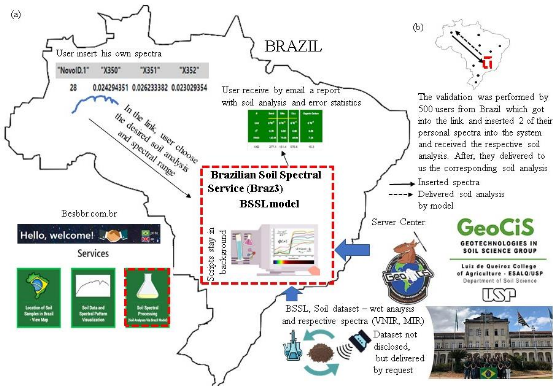
Figure 1. (a) How the system functions; (b) how the system was tested.
