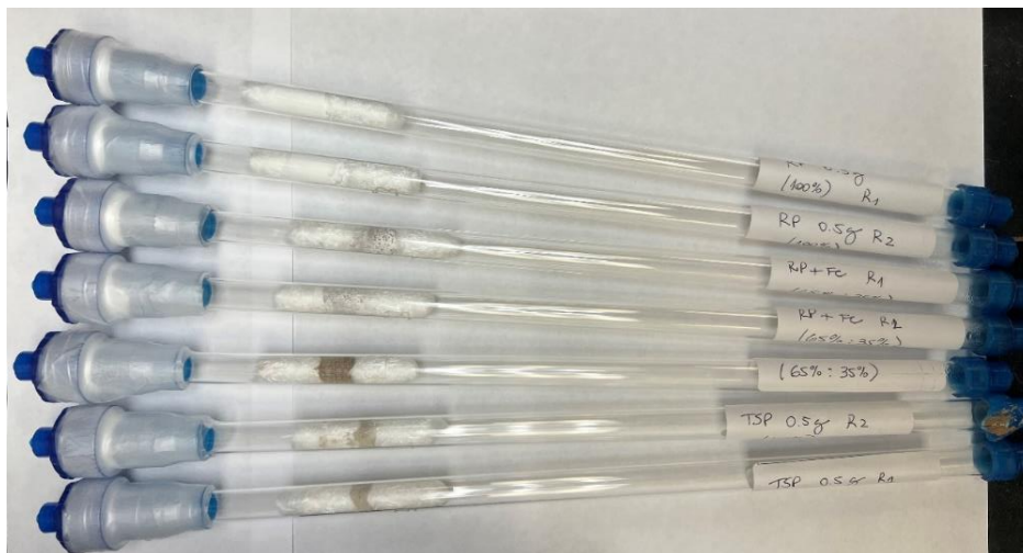
Figure S2. Grounded fertilizers – filter cake, triple superphosphate, triple superphosphate associated with filter cake, rock phosphate, and rock phosphate associated with filter cake -placed between nylon membrane filter and silanized glass wool in the glass columns (DWK Life Sciences Kimble Kontes FlexColumns™).
