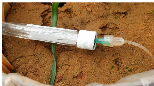
Figure S1. Soil solution recovered with Rhizon® (Rhizosphere Research Products, Wageningen, Netherlands) and sterile vacuum tube
