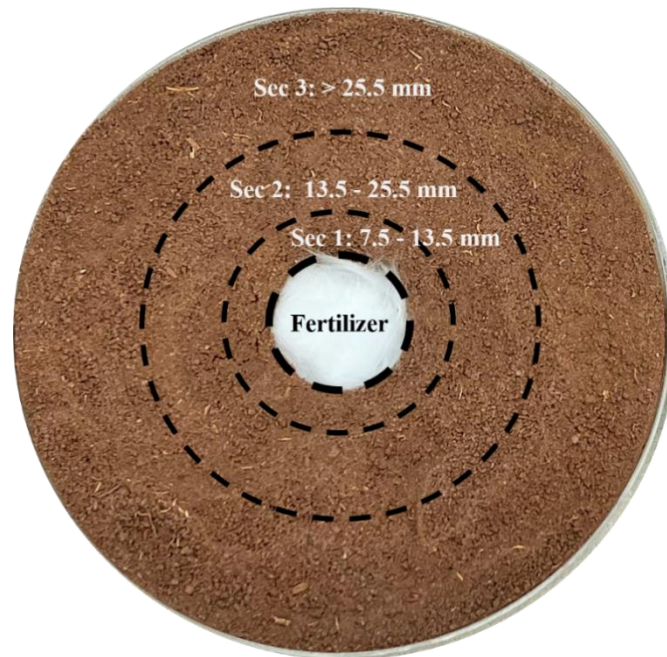
Figure S1. Representation of the fertilizer placed in the center of the Petri Dish, and the three soil sections sampled after 5 weeks of incubation.
