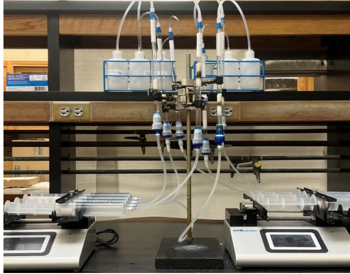
Figure S3. Setup of the column perfusion system used to evaluate the phosphorus release from fertilizers.
