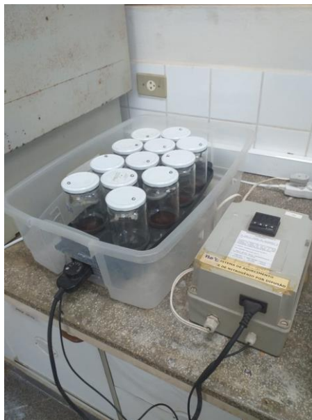
Supplementary Figure 4. Alkaline digestion in Mason jars heated in an electric hot plate (ISNT analysis).
