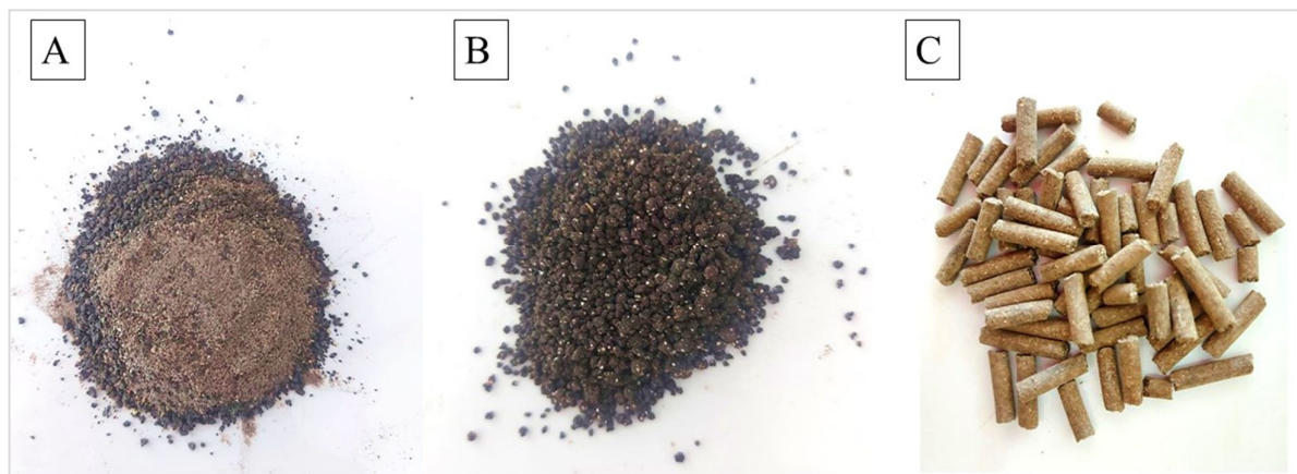
Fig. 3. Organomineral fertilizer from sewage sludge in the physical forms of powder (A), granule (B), and pellet (C).
