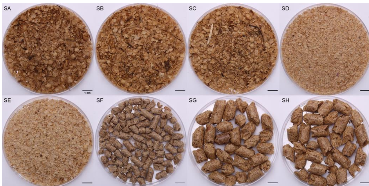
Figure 3. Visualization of the soybean hull samples. Note the different colors, particle sizes, and aggregation states: (SA-SE) loose hulls and (SF-SH) pelletized hulls
