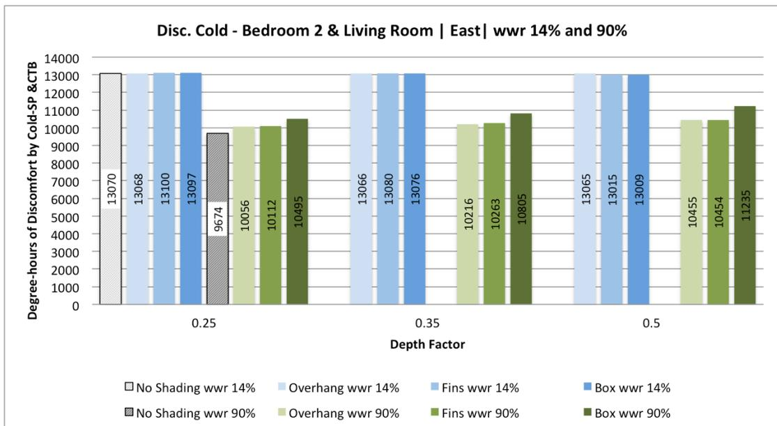
Figure 35 - Comparison of the Impact of Shading Devices with windows set with a WWR of 14% and 90% - Bedroom 2 and Living Room
