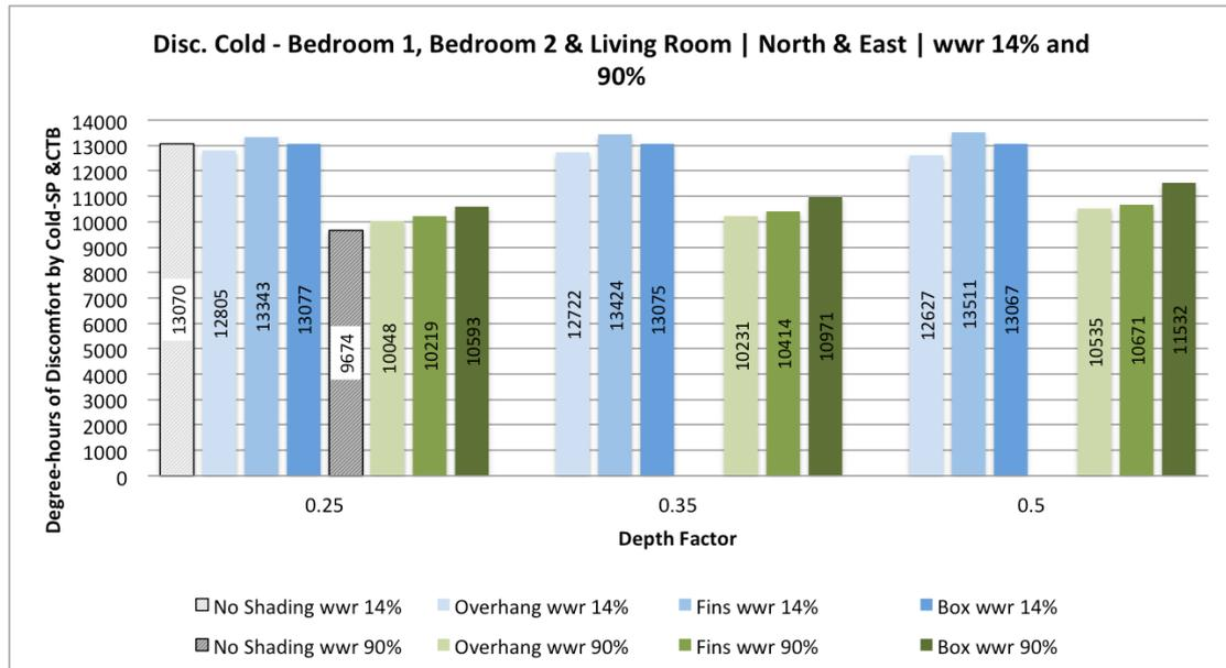
Figure 36 - Comparison of the Impact of Shading Devices with windows set with a WWR of 14% and 90% - All long-stay rooms
