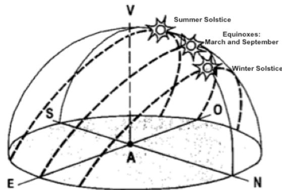
Figure 1 - Sun's trajectory and position at noon. Source: YANNAS; CORBELLA, 2003.
