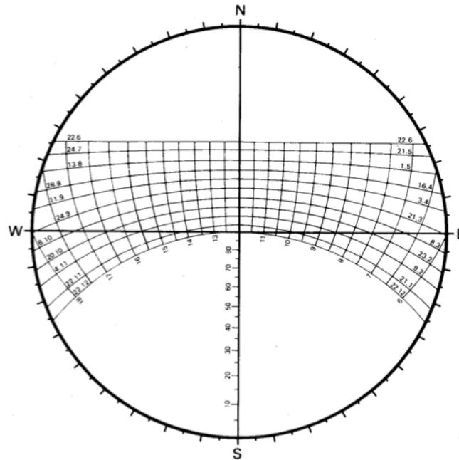
Figure 2 - Solar Chart for Latitude 24° South. Source: FROTA; SCHIFFER, 2001.
