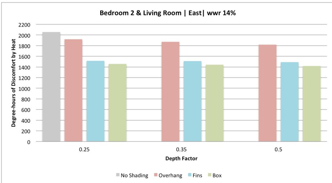
Figure 26 - Impact of Shading Devices when applied only to Bedroom 2 and Living Room facing East
