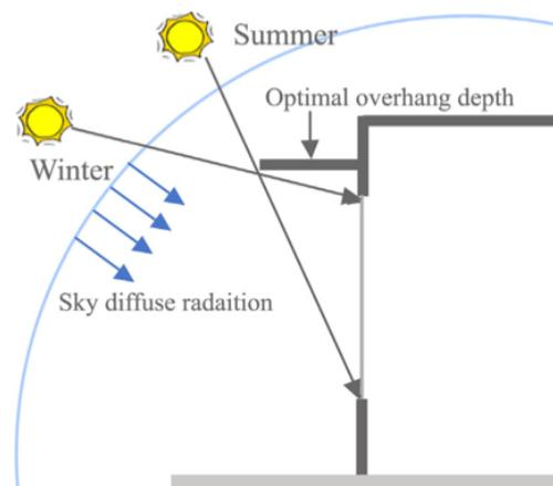
Figure 3 – Optimal overhang depth Source: Yao, 2014
