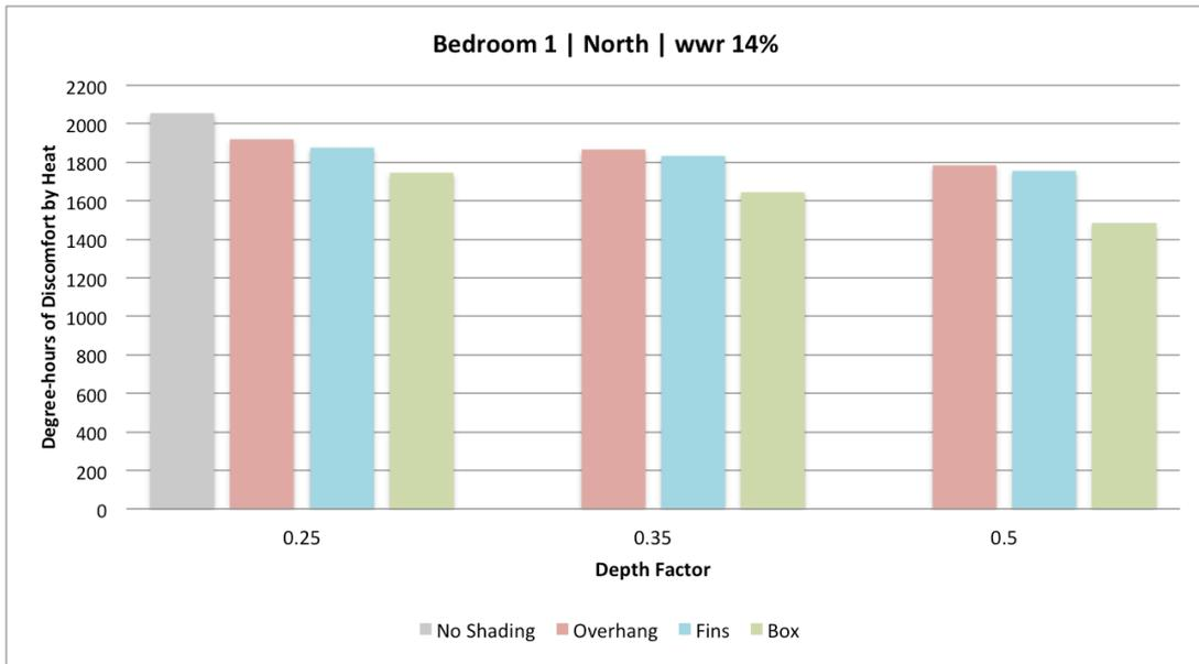
Figure 25 - Impact of Shading Devices when applied only to Bedroom 1 facing North
