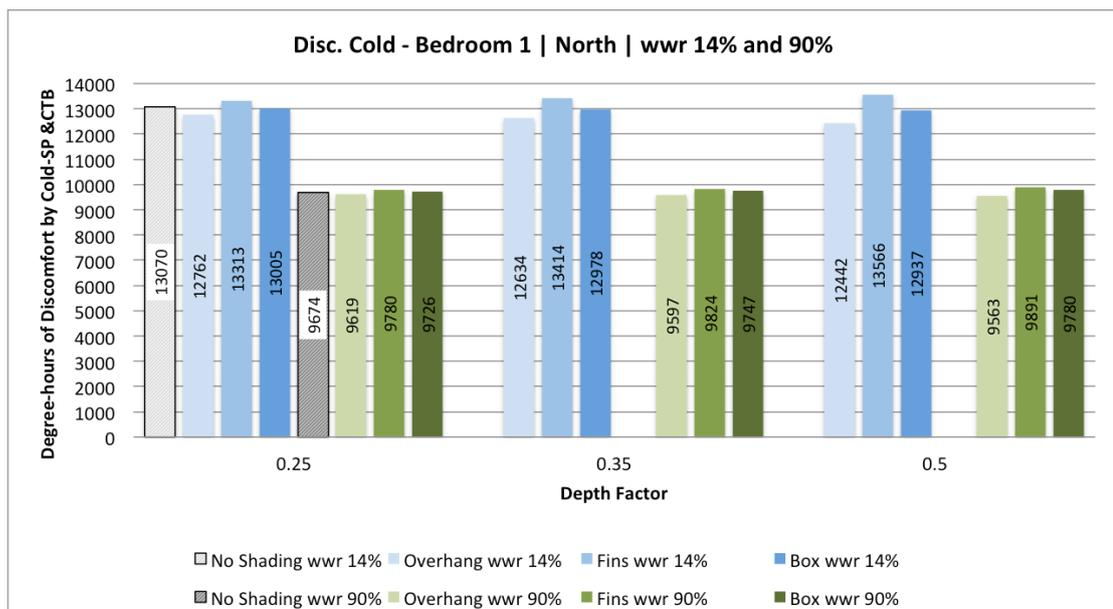
Figure 34 - Comparison of the Impact of Shading Devices with windows set with a WWR of 14% and 90% - Bedroom 1
