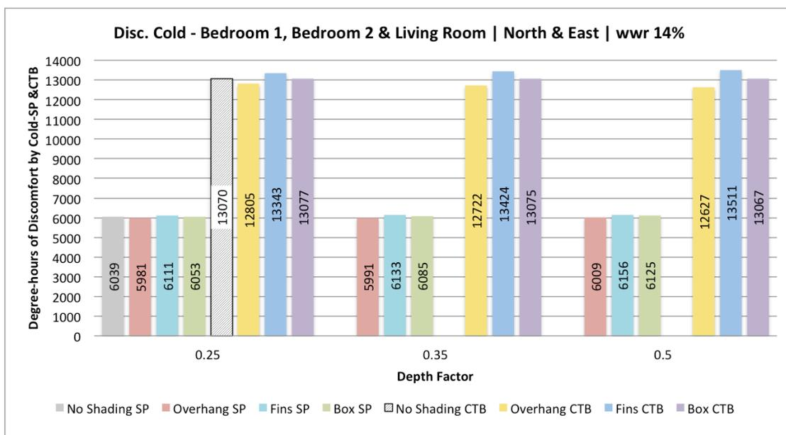
Figure 33 - Impact of Shading Devices in the Discomfort by Cold when applied to all long-stay rooms- São Paulo and Curitiba
