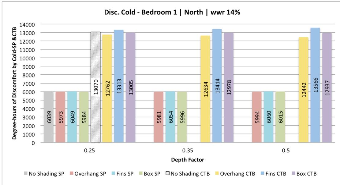
Figure 31 - Impact of Shading Devices in the Discomfort by Cold when applied only to Bedroom 1 facing North-São Paulo and Curitiba
