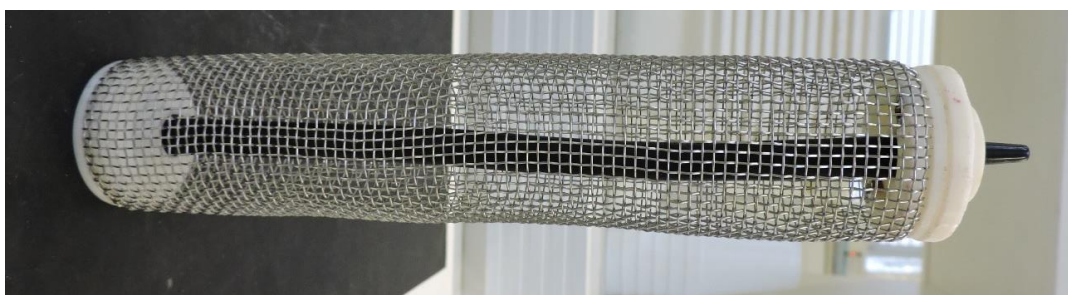
Figure 4.11 – Porous hose installed in the cathode grid chamber before filling it with GAC
