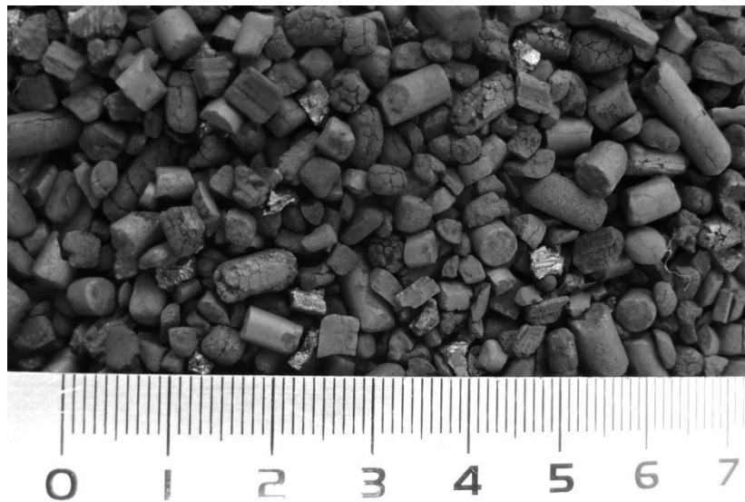
Figure 4.3 – Granular activated carbon used in the MFC
