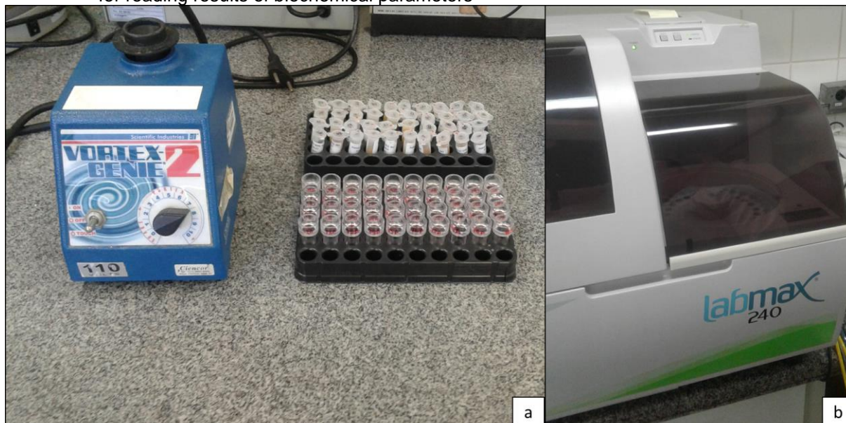
Figure 8 – Aliquots of samples pipetted on buckets of the automated biochemical analyzer and vortex utilized during the homogenization of the samples (a); automated biochemical analyzer used for reading results of biochemical parameters
