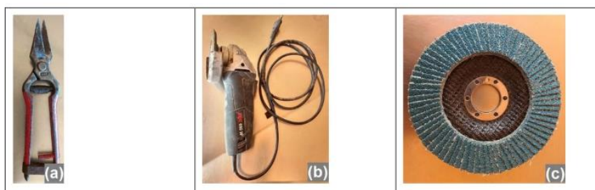
Fig. 1 Tools used for the two step claw trimming: (a) hoof shears for small ruminants; (b) angle grinder (c) sanding flap disc
