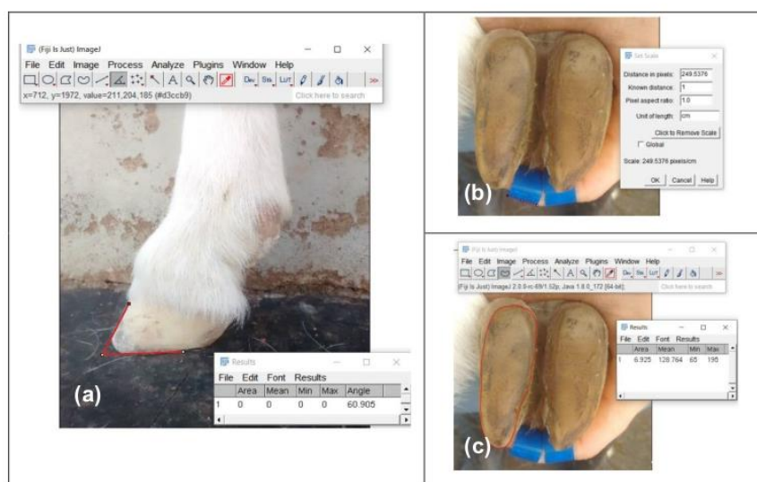
Fig. 3 Using the software Fiji/ImageJ (Schindelin et al., 2012), (a) the angle of the claw was measured using the Angle Tool that marked the required angle (red lines in the image), after three points were selected, providing its value in degrees, in the bottom box of the image. (b) To measure sole areas in \text{cm}^2 , through its photographs, the conversion rate from pixels to centimeters was established first. For this, the known width of a tape (1 cm) was selected in the image
