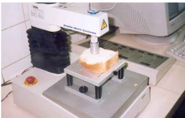
Figura 22. Texturômetro Texture Analyser TA-XT2i
