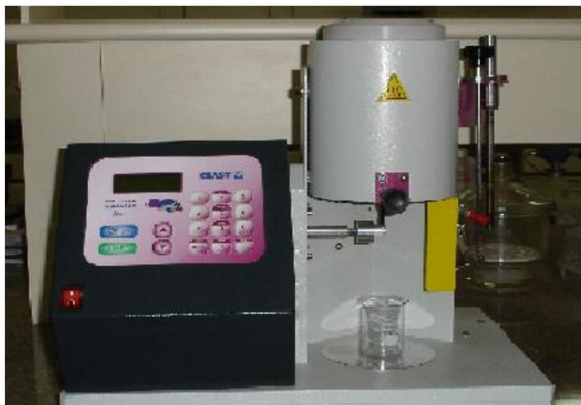
FIGURA 16. Plastômetro Modular Melt Flow, Ceast
