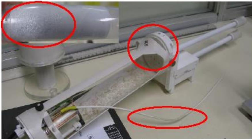
Figure 4 - Molten plastic coreholder and evaporation losses between the inside surface of the phial and the core sample wrapped up with synthetic tape.
