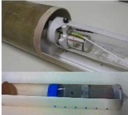
Figure 1 – Wrapped core sample with synthetic tape inside of the probe (top) and core sample inside of a phial of brine in the movable coreholder with acquisition marks (bottom).
