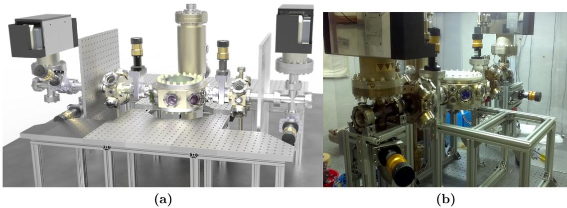
**Figure 3.1.2** – (a) and (b) show the experimental system with the optical table where the optical components are placed to produce the 3D-MOT, MT and BEC.
