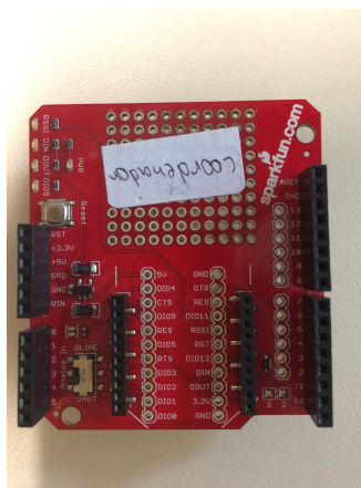
Figure 37 – Expansion shield to connect XBee to Arduino Leonardo photograph.
