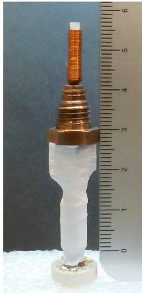
Figure 8.6: An example of pick-up coils to be used inside a pressure cell.
