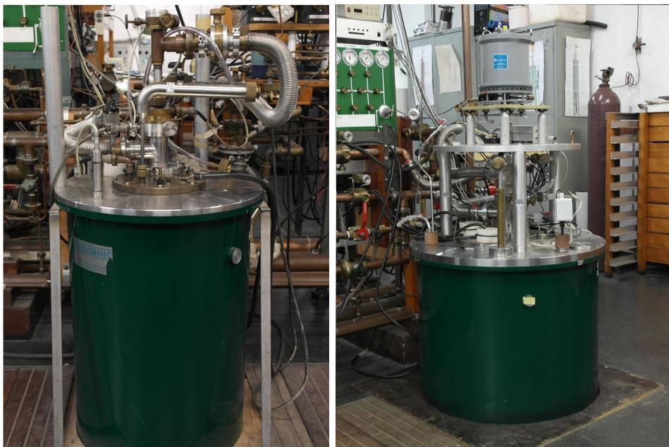
Figure 4.10: 7.5 T (left) and 20 T (right) cryostats.
