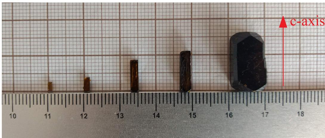
Figure 3.4: DTN samples of different sizes produced from the method of supersaturated solution. All the samples in the figure were align with the *c*-axis pointing vertically according to the red arrow.
