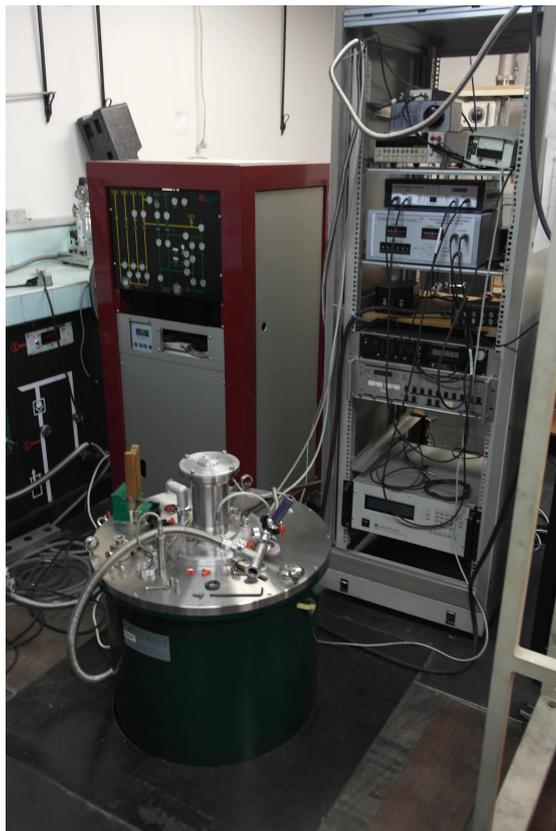
Figure 4.13: Cryostat with an ADR system to measurements of AC magnetic susceptibility at zero external magnetic field.
