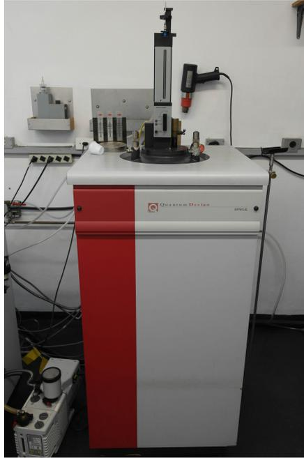
Figure 4.1: MPMS Model XL-7 SQUID magnetometer by Quantum Design used in our measurements.
