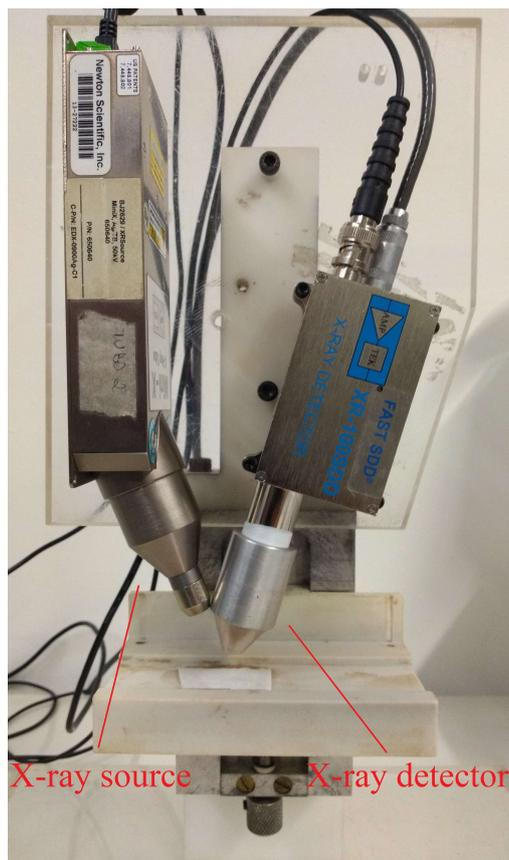
Figure 3.6: XRF setup used in this work with the X-ray source (on the left) and the X-ray detector (on the right).
