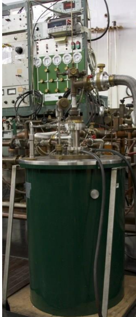
Fig.24 : 3-ac-susceptometer with 7.5 T superconducting coil and diffusion pumped He-3 glass cryostat for measurements down to 0.35 K.
