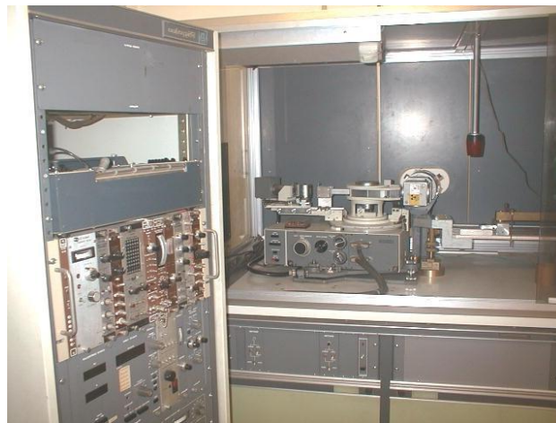
Fig.17: diffractometer theta-2theta, Bragg-Brentano geometry, at FAP (USP).
