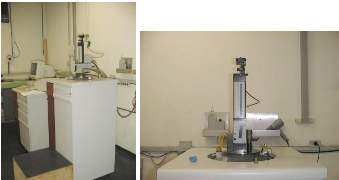
Fig.20 : 7 Tesla SQUID Magnetometer from Quantum Design (MSMS); 1.8 - 400K. AC & DC
