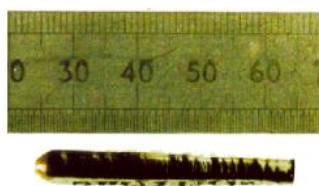
Fig.15: single crystal of the sample Sm 2 Ti 2 O 7 , with approx. 6cm of width and a diameter of 8-9mm, transparent to light with a deep red colour. [15]
