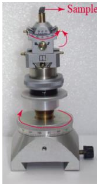
Fig.19: triple-axis goniometer used to find the crystal directions. The sample is placed in the indicated spot while the goniometer can be moved in the three indicated directions, with a high precision. Taken from the Crystal Growth Lab (DCMPMS, TIFR) page, from Mumbai, India.
