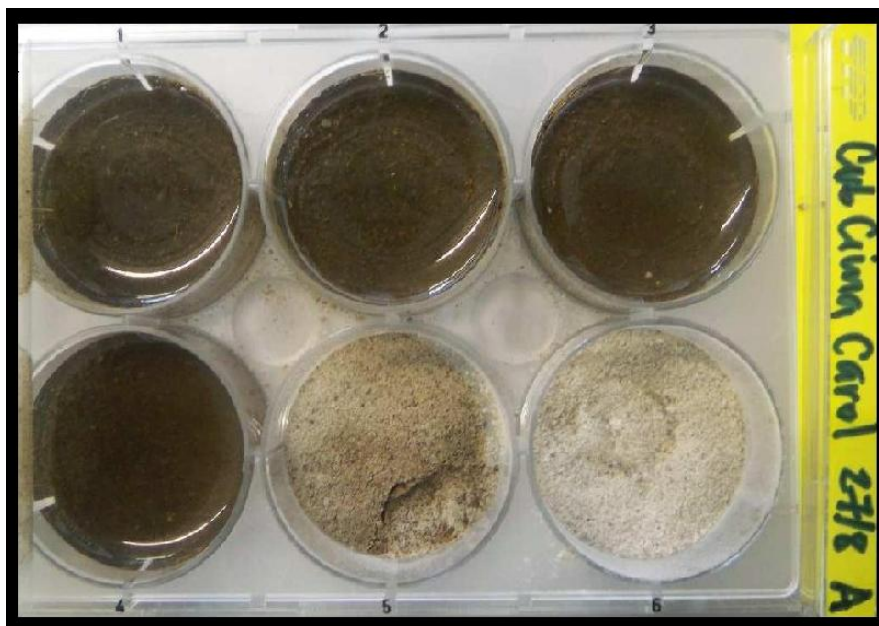
Figure 17. 6-well Plate with mixture of sediment and quartz sand, 5 mL of artificial water and 5 fish egg per well.
