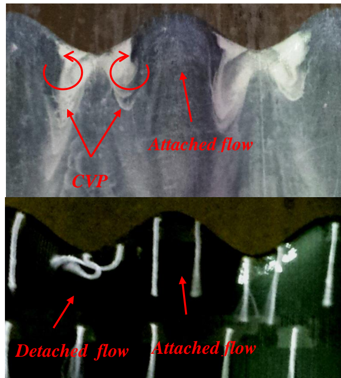
Figure 6.49: Vortical structures at greater amplitude-to-wavelength ratio ( A/\lambda ) (NACA 0012; A11 \lambda 40; \alpha = 10^\circ and Re = 290,000 ).
