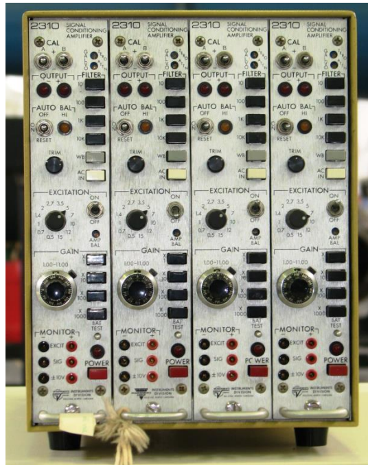
Figure 3.13: Signal conditioner used to amplify the bridge's output signal.
