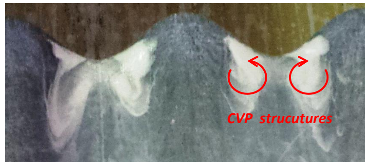
Figure 6.42: Counter-rotating vortex pair (CVP) at wavy airfoil (NACA 0012; A11\lambda40 ; \alpha = 10^\circ and Re=290,000 ).
