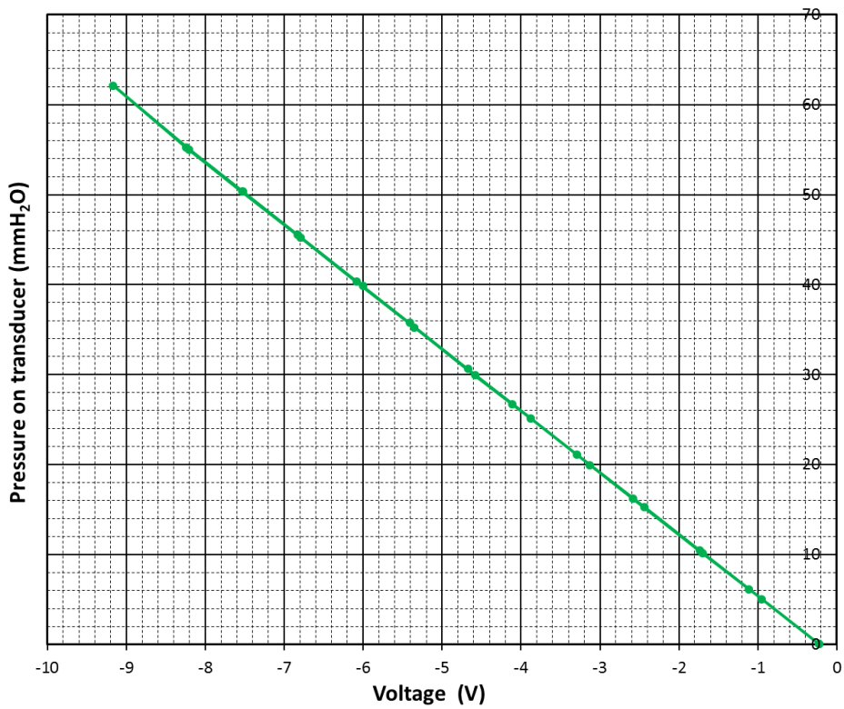
Figure 3.19: Calibration curve of the pressure transducer (Dynamic pressure).
