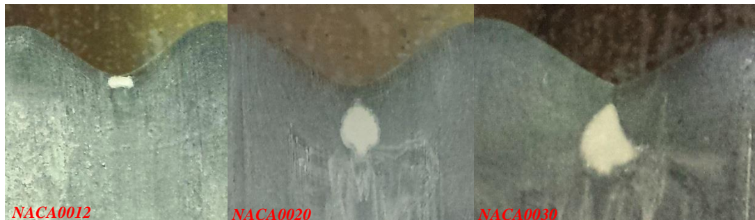
Figure 6.18: The leading edge radius effect on flow topology at A11 \lambda 40 wavy airfoil ( \alpha = 5^\circ and Re = 290,000 ).
