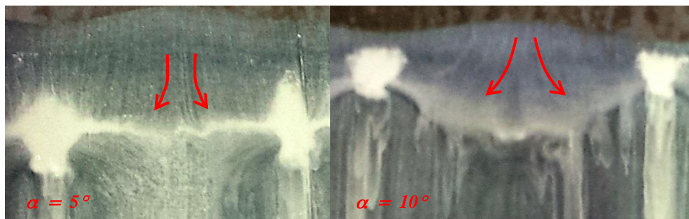
Figure 6.16: The raise in streamline deflections along span with increasing of angle of attack indicating increase in streamwise vorticity.
