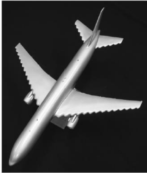
Figure 1.11: The tubercles replacing high lift devices needs decreasing weight and maintaining cost (FISH, 2011).
