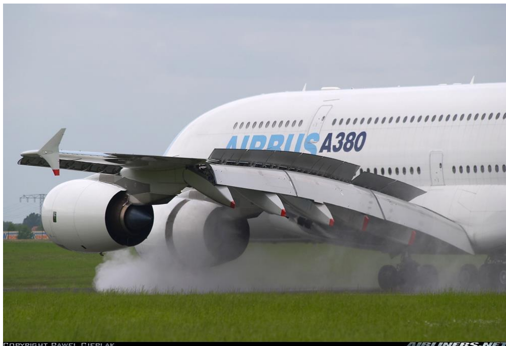
Figure 1.1: Modern high lift devices deployed during the landing of the aircraft Airbus 380. Reproduced from http://www.airliners.net/photo/Airbus/Airbus-A380-841/1062608/L/ .
