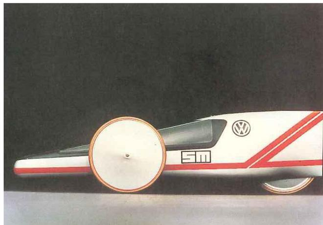
Figura 12-7: Volkswagen “Sparomobil”,  $C_D = 0.15$ ,  $A = 0.32 \text{ m}^2$  (HUCHO, 1998, p. 234).
