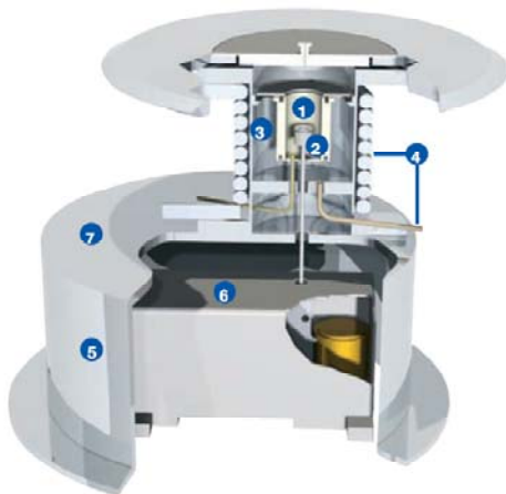
Figure 64 – Perkin Elmer Simultaneous Thermal Analyzer (STA) 6000 for TG, DTG and DSC analysis.
