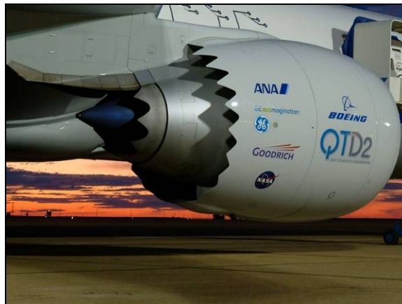
Figure 2.10 - Chevrons installed on the engine and nacelle from a Boeing 787 aircraft. 6
