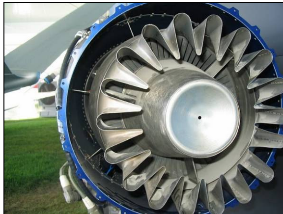
Figure 2.11 - The back end of a Williams FJ-33 turbofan showing the application of the mixer for jet noise reduction. 7
