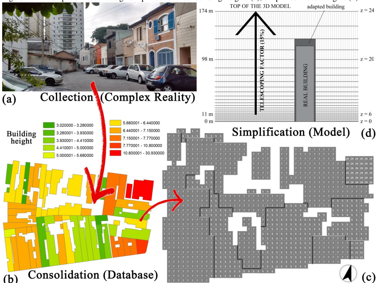
Figure 17 – Example of model design simplification: real building heights (a), simplified model heights (b).
