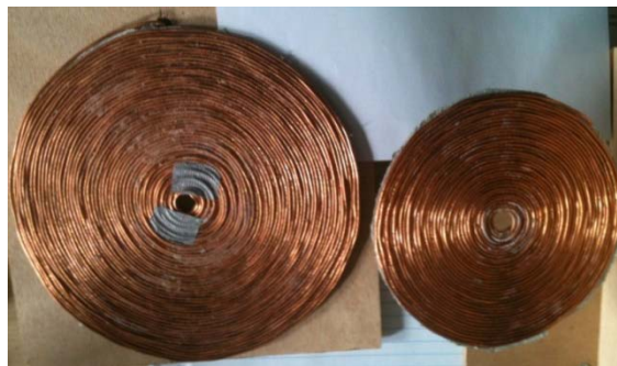
Figure 3.20 – Built coils with wire AWG 15.
