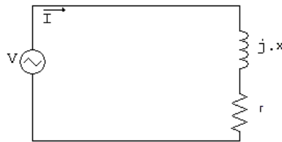
Figure 3.3 – Equivalent circuit of one coil separately.
