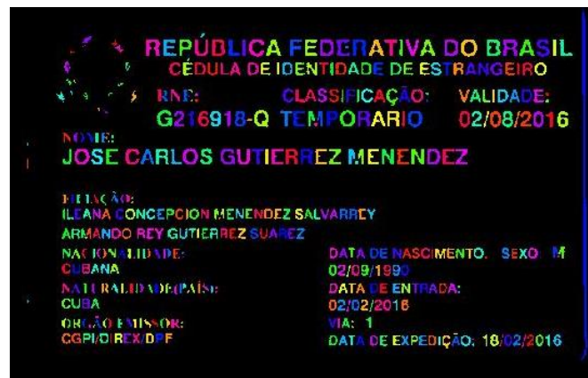
Figure 2-7 Connected components obtained using an 8-connectivity. Each color represents a component. Source: The Author
