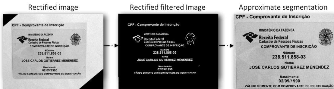
Figure 4-5 From the rectified filtered image, it is assumed that the regions of interest are in the area where the greatest amount of information with similar sizes is concentrated. Therefore, the image is cropped to only contains the information of interest. Source: The Author.
