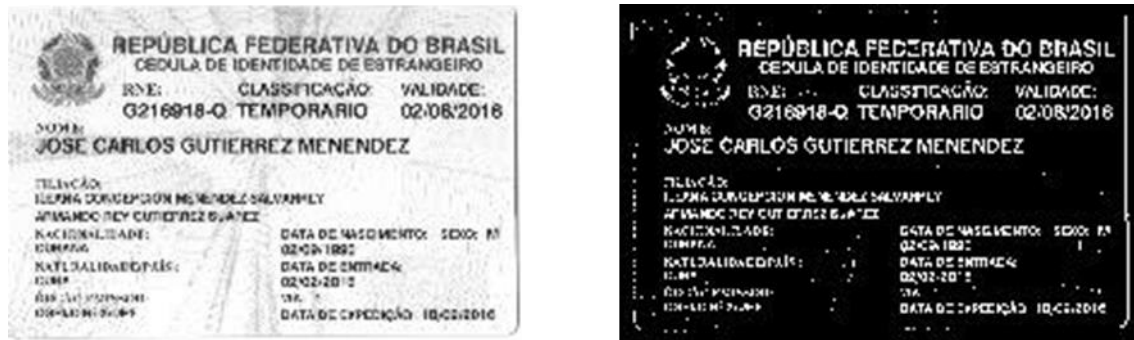
Figure 2-6 Result of applying an adaptive threshold operation over an image with text. Source: The Author.
