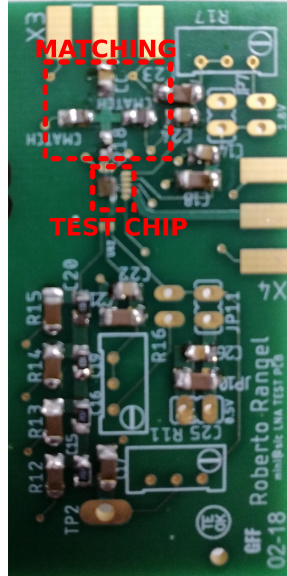
Figure 26: Fabricated test PCB for the LNA and Buffer circuit.
