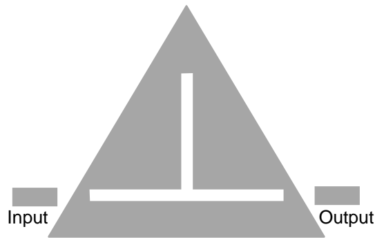
Figure 13 – Layout of the triangular patch resonator weakly coupled to the input and output, with a vertical and a horizontal slot.
