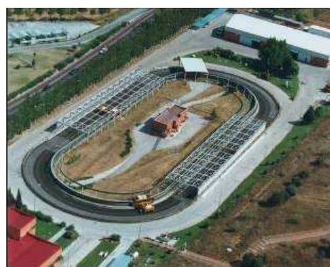
Figura 51 - Linear test track - CEDEX Madrid - http://www.cedex.es/apt2008/html/docs/apt_update/Spain_CEDEX
