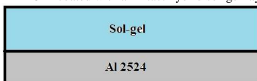
Figure 5.20 - Physical model of the non-anodized AA2524 coated with an intact hybrid sol-gel layer.
