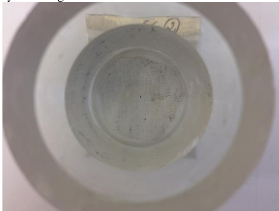
Figure 5.19 - Photograph of non-anodized AA2524 coated with the hybrid sol-gel after 72 h of immersion in 0.1 \text{ mol.L}^{-1} NaCl.
