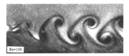
Figure 6.2: The laminar and two-dimensional vortex shedding at Re = 150 (WILLIAMSON, 1996).
