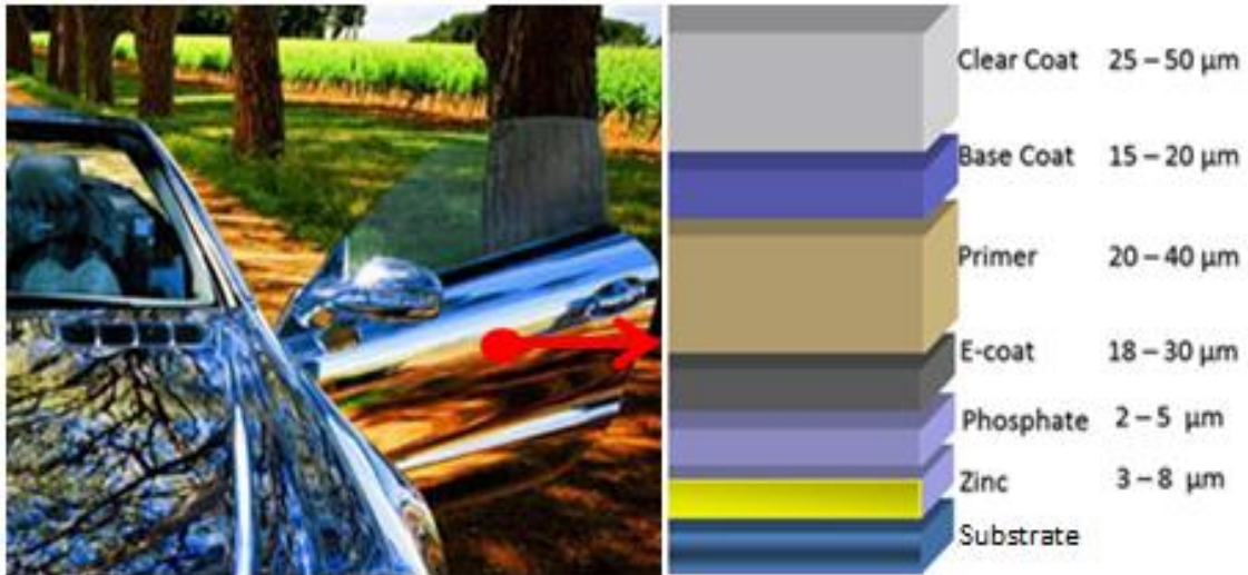
Figure 3.3.1: The layers: from substrate to clear coat (LEX, 2010).
