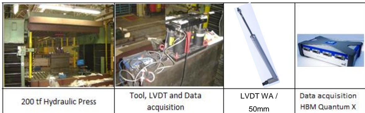
Figure 4.4: Equipment used in the second run, first step. Technical details (for each equipment), are given in the attachment 2.
