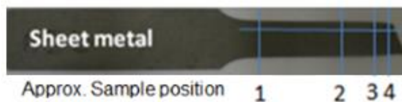
Figure 6.2.8: Approximately sample position for 2D and 3D roughness measurements.
