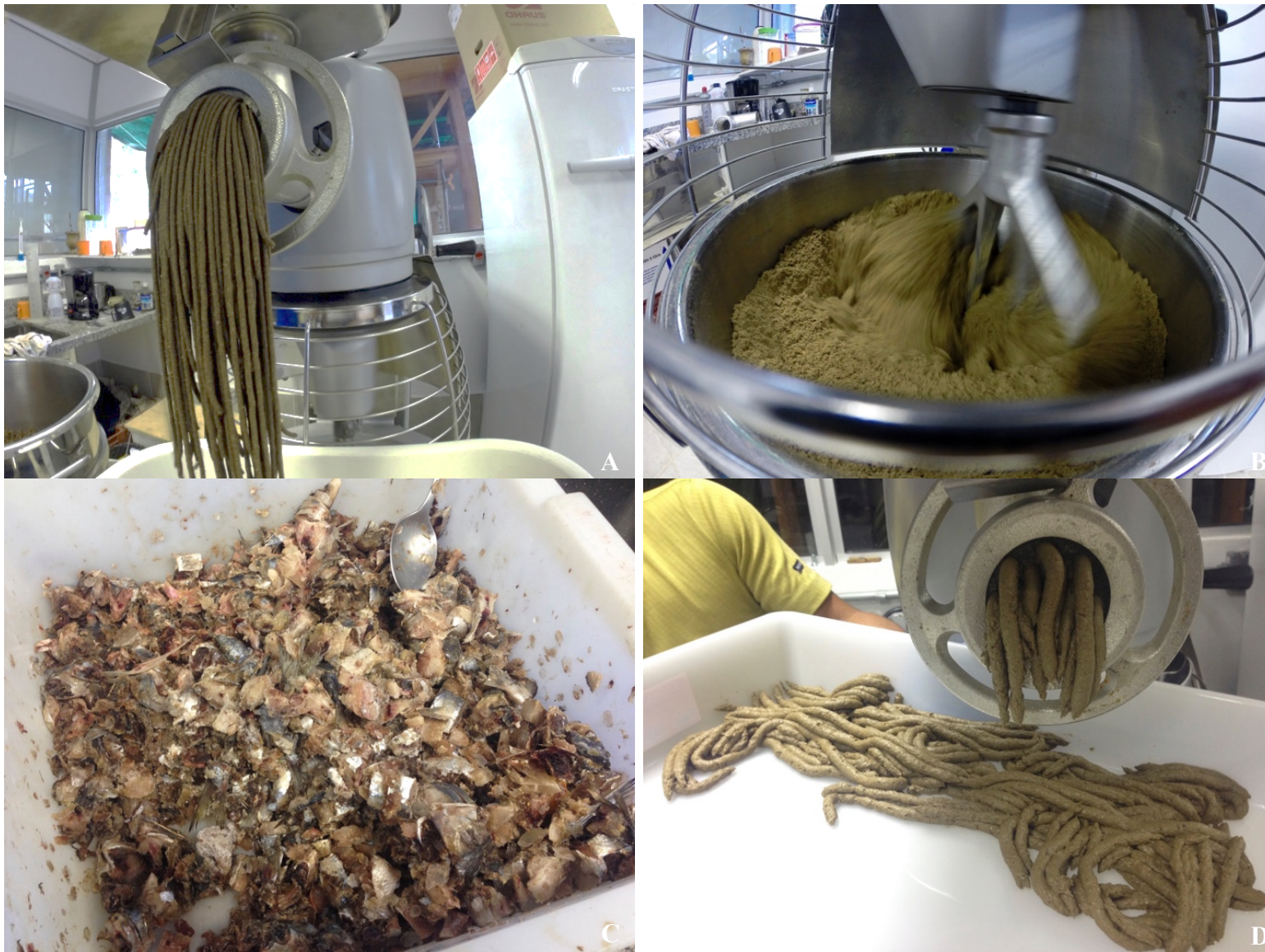
Figure 9 Feed preparation: ingredients were homogenized in an industrial food mixer (A); and cold-pelleted through a 3-mm die (B); trash-fish were bought from local fishing boats (C); finished semi-moist feed prepared by mixing the Aquamar diet (60%) with trash-fish (40%)(D).
