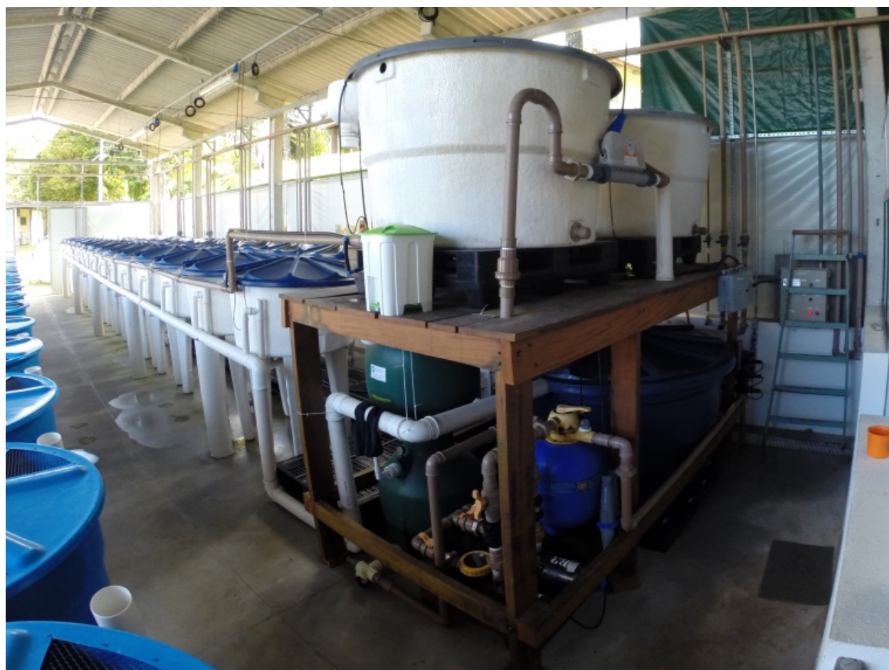
Figure 3 Overview of the closed recirculating system used for the digestibility trial with juvenile shrimp.
