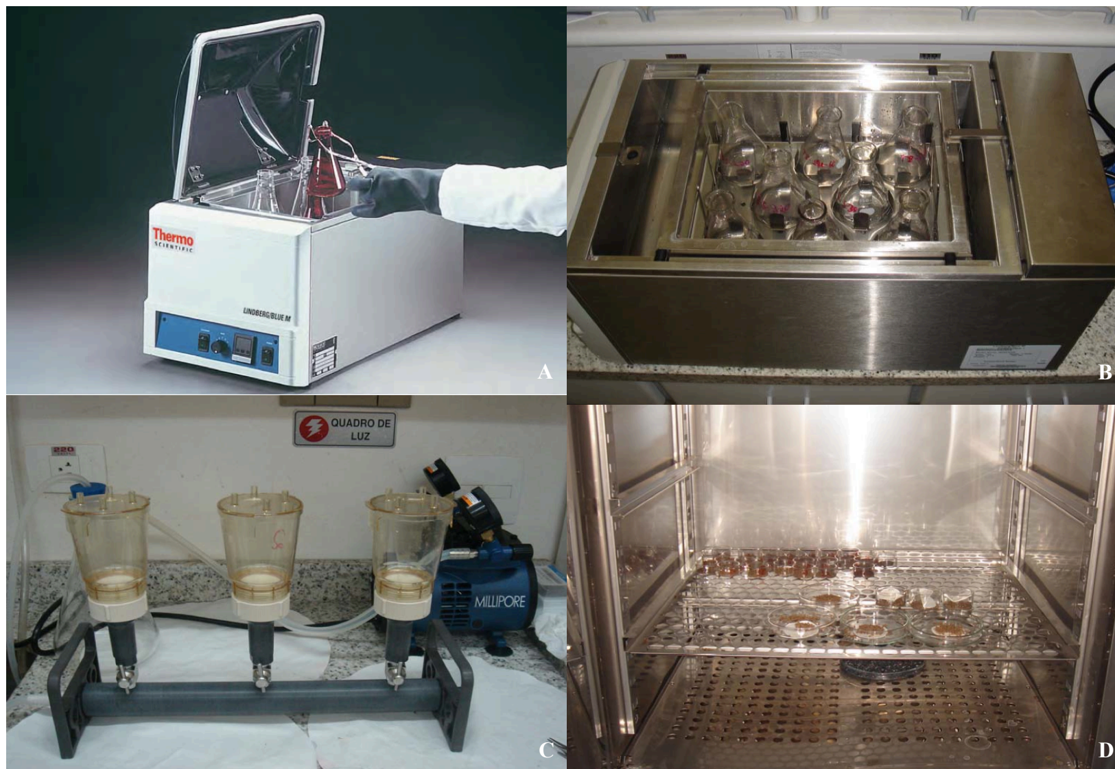
Figure 7 Equipments used for the pellet water stability applying the water bath apparatus: refrigerated shaking water bath (A), 250 mL flasks (B), filtration apparatus with filter (C). Dry recovered and original feed samples in the oven at 105°C for 24h (D).
