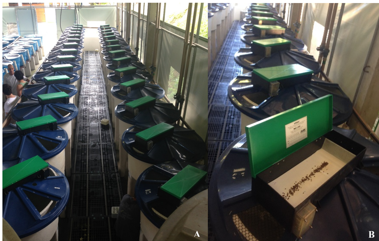
Figure 2 Shrimp digestibility system adapted from the original system according CARVALHO et al. (2013) (A). View of the automatic belt-feeder loaded with feed (B).
