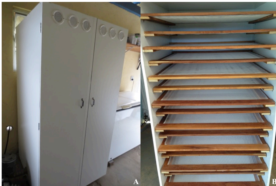
Figure 11 Drying cabinet built using an air blower at 38°C (A). View of the cabinet shelves accommodated alternately in order to let the air to flow and exit through the holes on top of the doors (B).
