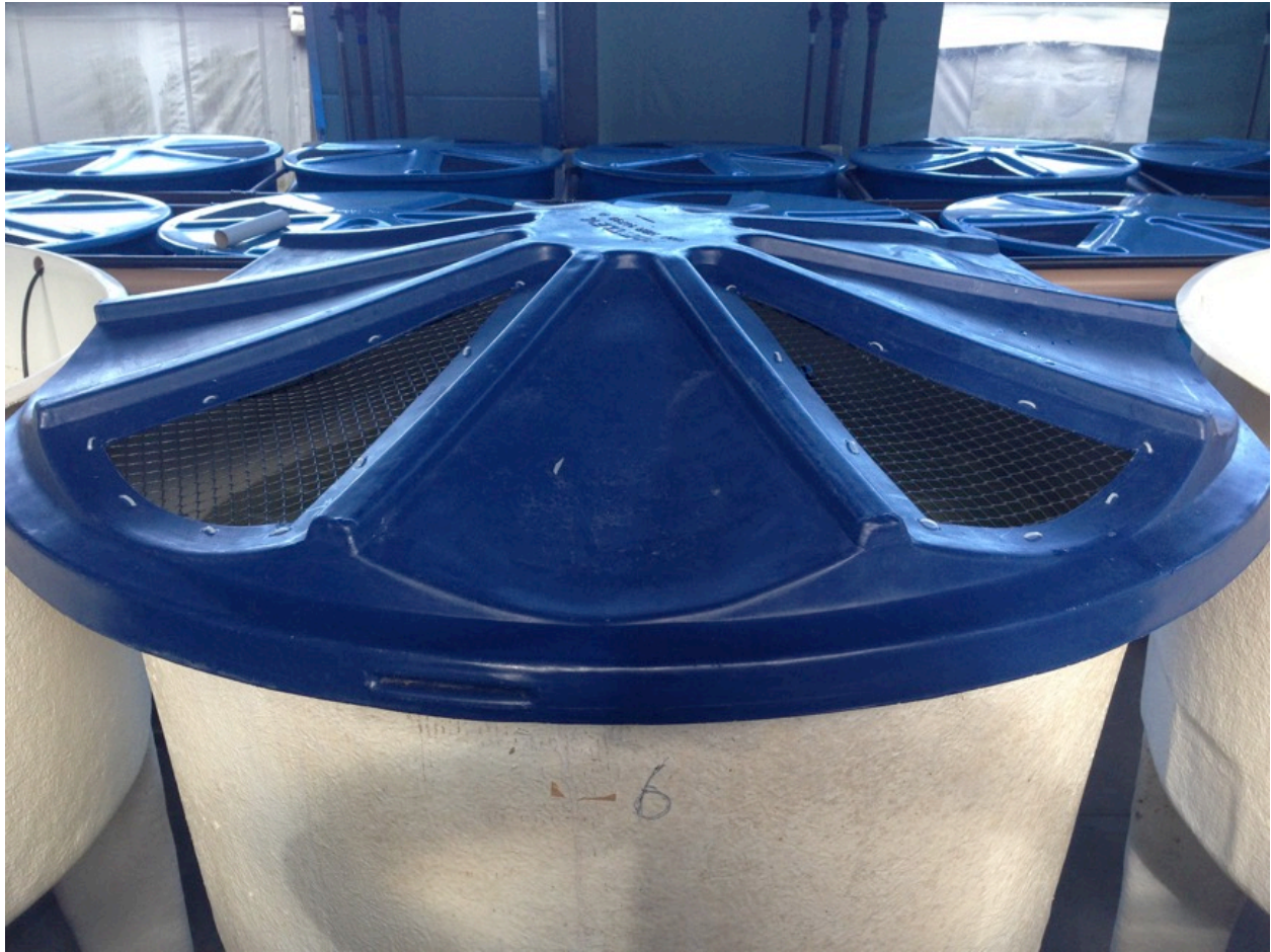
Figure 6 Polyethylene covers to reduce heat loss to the external environment, prevent the escape of animals and decrease lighting intensity inside the tanks.
