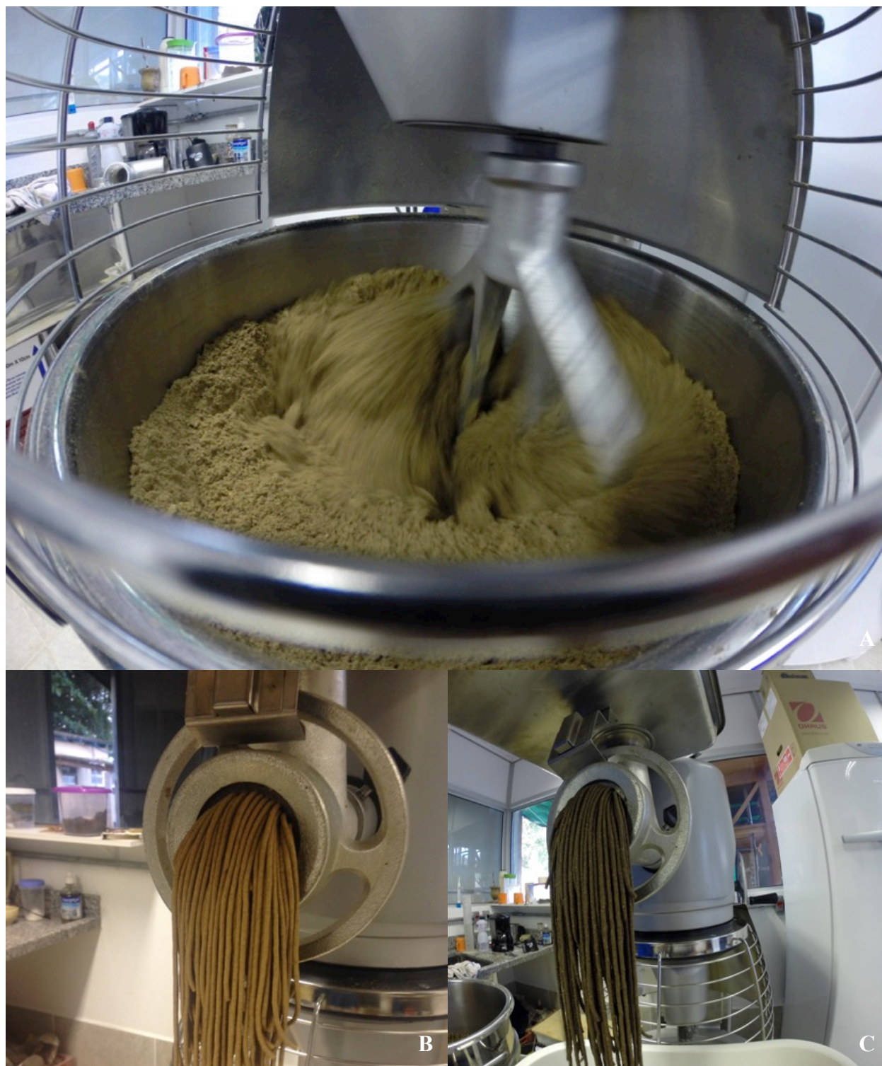
Figure 9 Industrial food mixer (A) used to blend the ingredients and cold-pellet the diets. Commercial mixture being cold pelleted (B); commercial mixture being cold pelleted with addition of the external marker chromic oxide (C).
