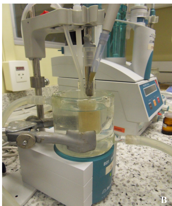
Figure 8 Ready-to-use enzymes (A). Simulation of shrimp and fish digestion in a pH-stat assay: reacting vessel kept temperature stable in glass jacket (B); potentiometric titrator (C).
