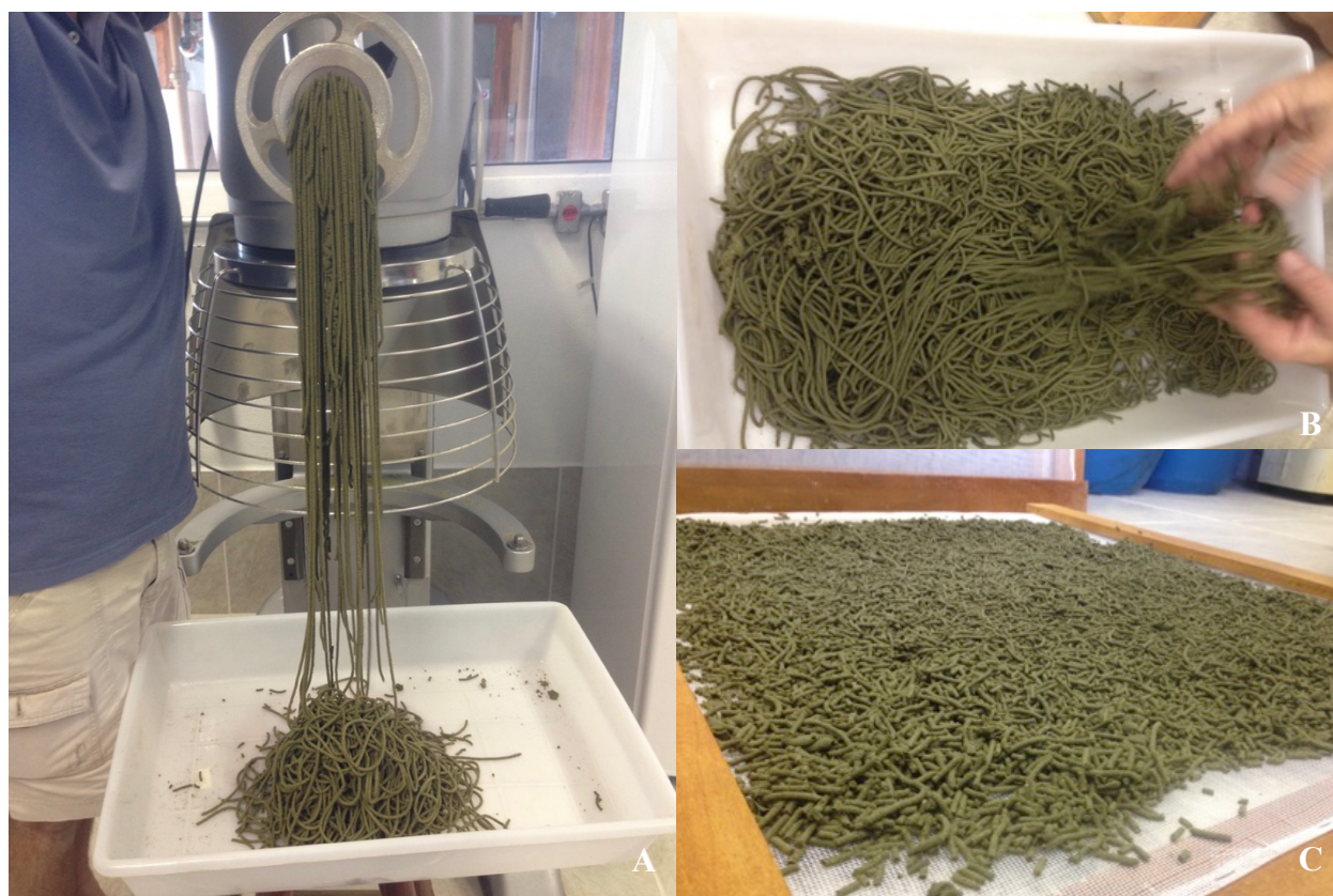
Figure 13 Moist pellets feed being prepared in the industrial mixer (A), which were then scattered and manually broken into smaller pieces (B). The feed was placed over the dryer shelf, and then dried overnight until the moisture level was between 6.5-7.5% (C).
