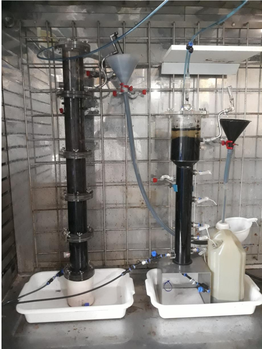
Figure S. 5. Experimental setup. 1 st -stage reactor (left) and 2 nd -stage reactor (right) operated in series.
